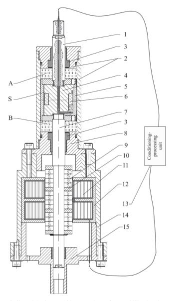
Fig. 2. Structure of a linear MR damper with energy harvesting capability: 1 – piston rod; 2 – damper housing; 3 – sleeve; 4 – piston core; 5 – piston ring; 6 – damper coil; 7 – transducer stem; 8 – connecting lid; 9 – permanent magnets; 10 – pole pieces; 11 – transducer coil; 12 – transducer coil housing; 13 – signal conditioning-processing system; 14 – transducer frame; 15 – transducer cover; S – slit, A, B – space filled with MR fluid
