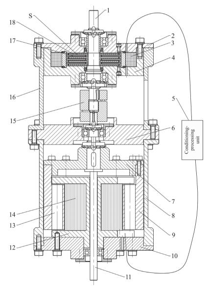
Fig. 3. Structure of a rotary MR damper with energy harvesting capability: 1 – shaft; 2 – damper lid;
