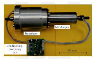
Fig. 4. Linear MR damper with energy harvesting capability - general view
