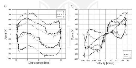
Fig. 6. Characteristic of a linear MR damper with energy harvesting capability: a) force vs displacement, b) force vs velocity
