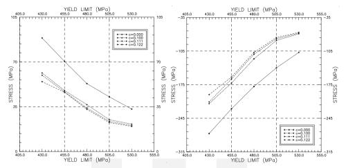
Fig. 7. Peak longitudinal residual stress, vs. yield limit, tension (left) and compression (right); c = 0.0 – perfect plasticity
