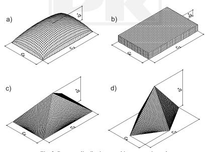
Fig. 3. Pressure distributions used in parametric study
