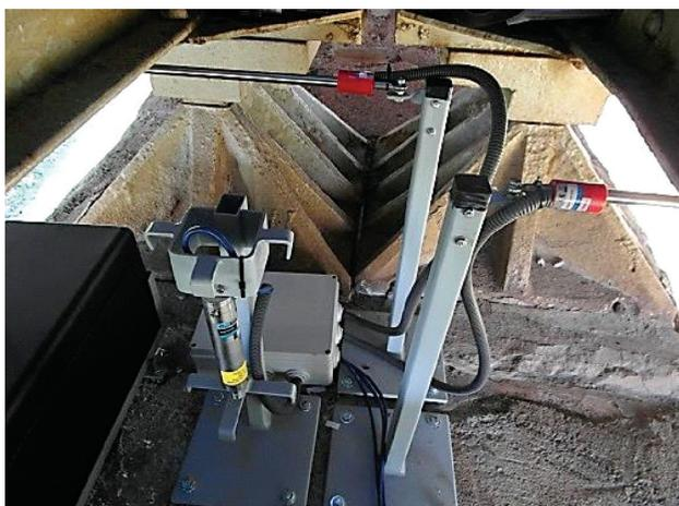
Fig. 5. Support structures for mounting angle sensors and displacement sensors at the intermediate support (view on the west side)
