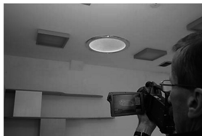
Fig. 6. Detection of leakages with infrared camera
