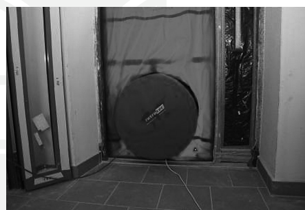
Fig. 2b. Blowerdoor set –internal view
