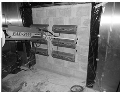
Fig. 4. Heating surface of the test wall by infrared radiators with power 7,2 kW
