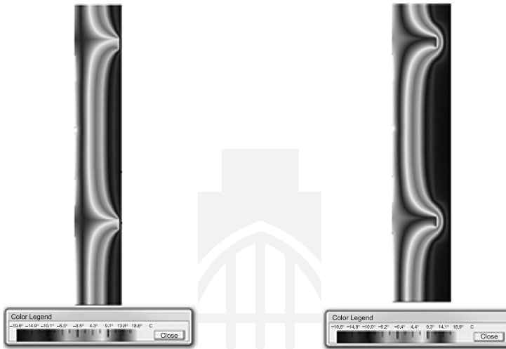
Fig. 3. Calculation results of a wall panel – temperature field distribution in wall's cross-section, standard (left) modified (right)
