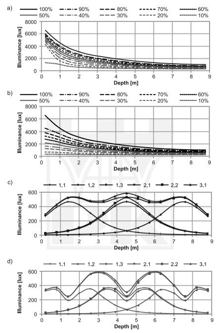
Fig. 2. Interior illuminance for different: a) size of the window, b) visible transmittance of the window, c) position of 0.85 m diameter light pipes with transparent diffuser, d) position of 0.85 m diameter light pipes with matt diffuser
