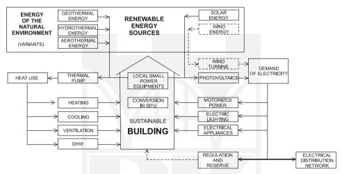
Fig. 4. Scheme of sustainable building with zero energy balance in relation to the distribution networks (net zero energy sustainable building). It has zero requirements of the energy demand for heating, cooling, ventilation and domestic hot water preparation and also zero requirements of the energy for motor drives, electric lighting and appliances. It is, in terms of the regulation and the reserve, always connected to the distribution network of electric energy
