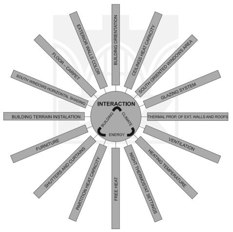
Fig. 2. Building in the system building – climate – energy is defined by the subsystem factors influencing its annual energy consumption
