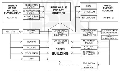
Fig. 3. Scheme of green building with nearly zero energy balance in relation to the distribution networks (nearly net zero energy green building). It has zero requirements of the energy demand for heating, cooling, ventilation and domestic hot water preparation from the distribution energy network
