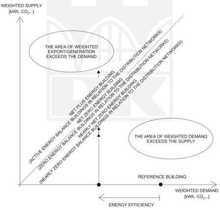
Fig. 1. Scheme of graphic dependence representing a way towards zero energy buildings in relation to the distribution network with alternatives "nearly" and "active"
