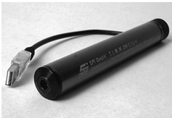
Fig. 6. An optical video microscope used for detecting fissures in wheel webs
