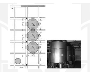
Fig. 3. The proposed schema of location tanks. View of the tanks positioned on the slab
