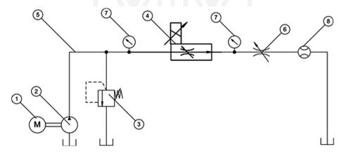
Fig. 2. General diagram of the power supply system and flow controller
