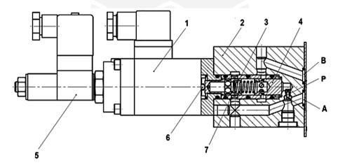
Fig. 1. Diagram of two-way proportional flow control
