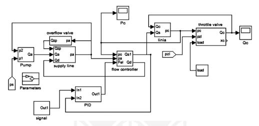
Fig. 5. Block diagram of the hydraulic system was built in Matlab - Simulink
