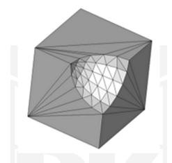
Fig. 4. 3D model surface saved in STL format [2]
