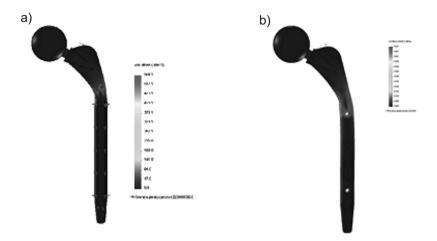
Fig. 2. Distribution of stresses in the hip joint endoprothesis for different kinds of boundary conditions
