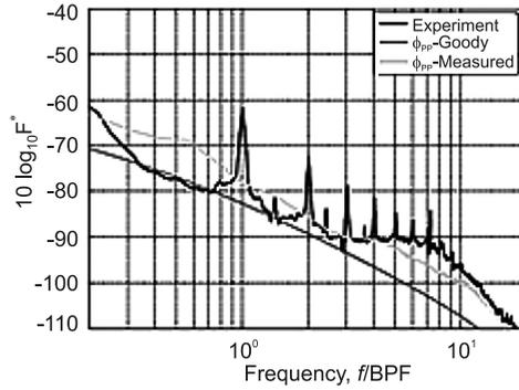
Fig. 7. Comparison of spectral acoustic densities determined by Goody model and experiment [13]
