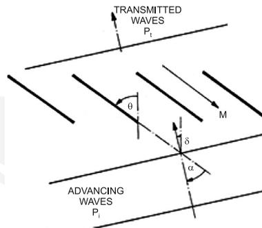
Fig. 6. The method of inlet guide vane attenuation [12]
