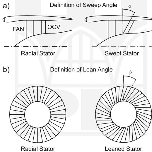
Fig. 8. The swept and leaned stator concept [4]
