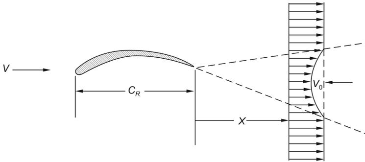
Fig. 2. Model of the rotor wake velocity defect [2]
