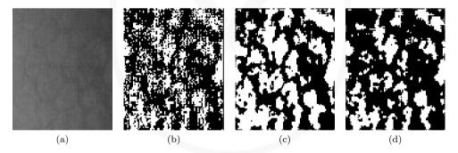
Fig. 4. Adaptive binarization results. The source image (a) processed without the median filter (b), with the median filter and the 55% (c) and 60% threshold
