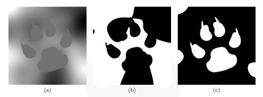
**Fig. 1.** An example of bad and good binarization. The source image has a low dynamic range (a) and auto threshold binarization gives poor results (b). The required effect is presented in the image (c)
