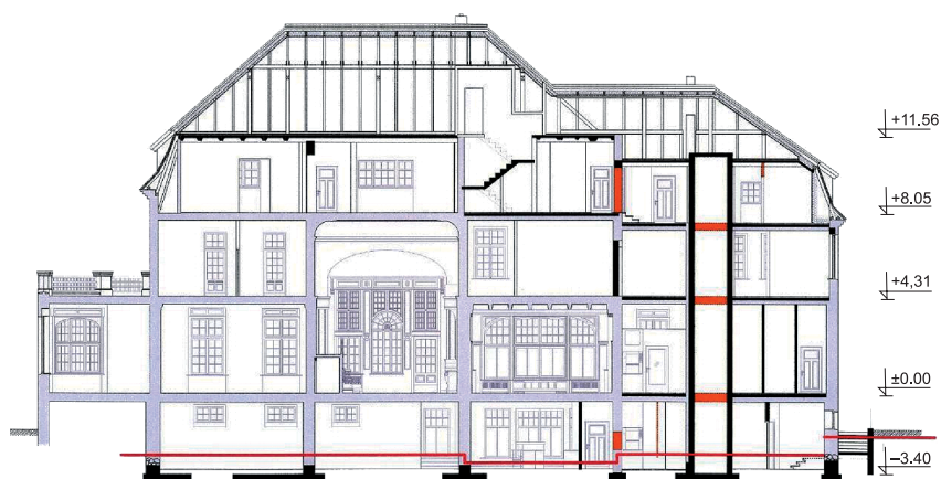
Fig. 19. Longitudinal section of the Villa Casablanca, 2010. The red line indicates the cellar floor level before the deepening of the basement
