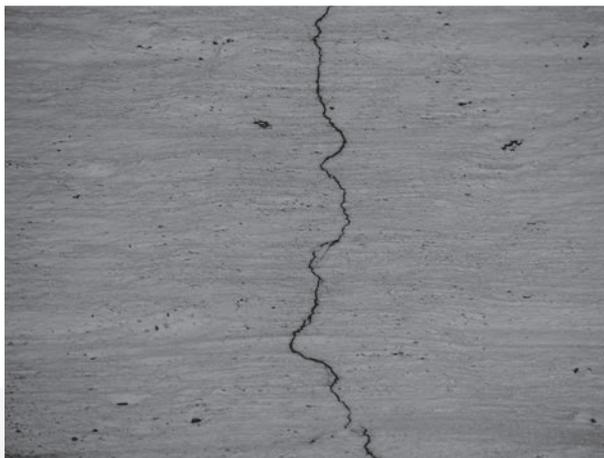
Fig. 2. Crack on the head surface
