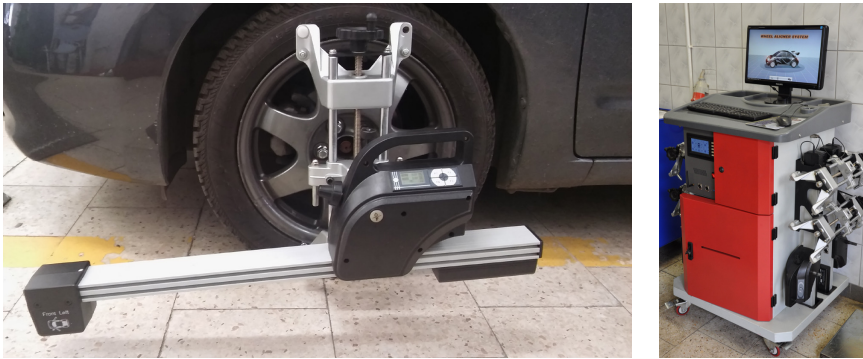
Fig. 2. An overview of the CUSTOR HWA G58 wheel alignment device and a close-up of a front left head attached to the wheel
