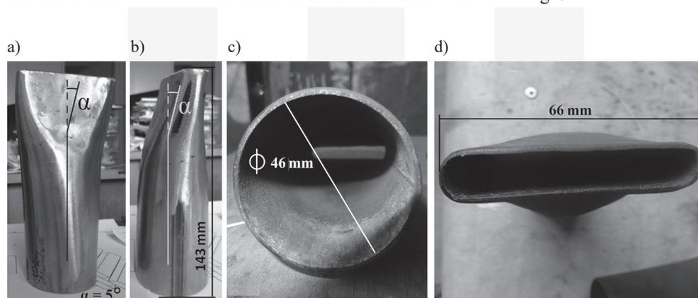
Fig. 4. Nozzles, which are responsible for deflection of the secondary air fluxes in the experiment
