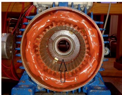
Fig. 2. View of the examined motor stator with the installed coil for measuring the axial flux
