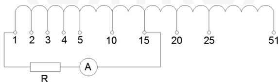
Fig. 1. Diagram of routed-out turns from one of the modified coils of stator windings
