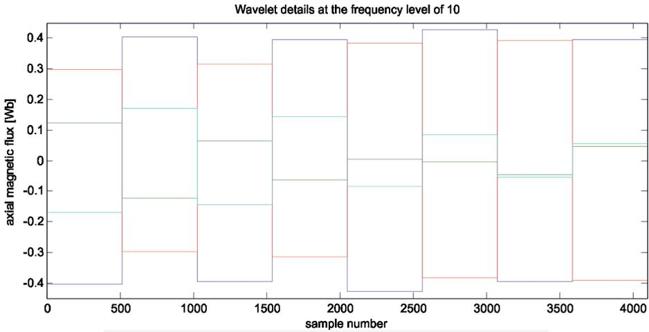
Fig. 6. Wavelet details of axial magnetic flux signal at the frequency level of 10 [D10 – colours: navy blue – symmetrical motor; green – short circuit 1–2; red – short circuit 1–3; blue – short circuit 1–4]
