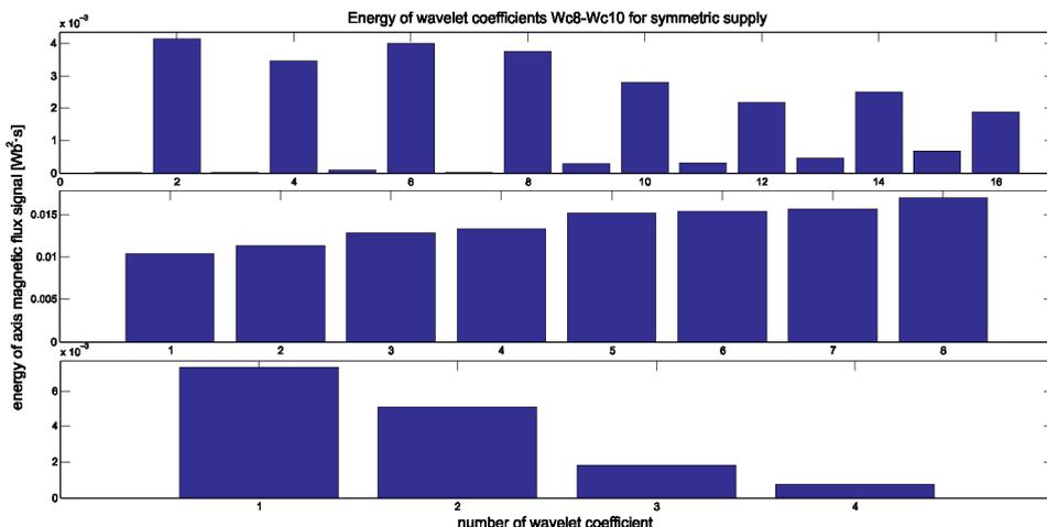
Fig. 8. Energy of wavelet coefficients of signal proportional to axial magnetic flux for the most important levels of wavelet representation from 8 to 10 – the case with symmetrical supply
