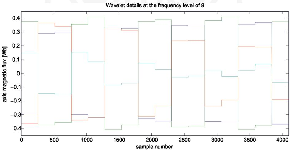
Fig. 5. Wavelet details of axial magnetic flux signal at the frequency level of 9 [D9 – colours: navy blue – symmetrical motor; green – short circuit 1-2; red – short circuit 1-3; blue – short circuit 1-4]
