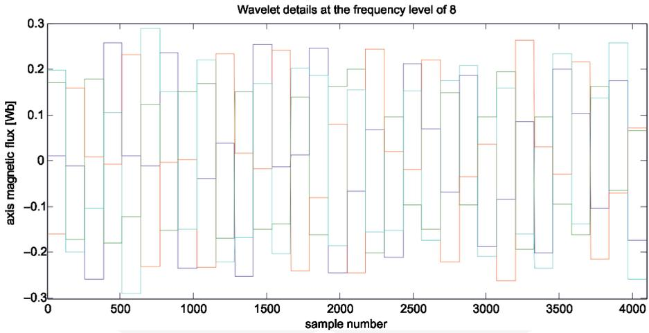
Fig. 4. Wavelet details of axial magnetic flux signal at the frequency level of 8 [D8 – colours: navy blue – symmetrical motor; green – short circuit 1-2; red – short circuit 1-3; blue – short circuit 1-4]
