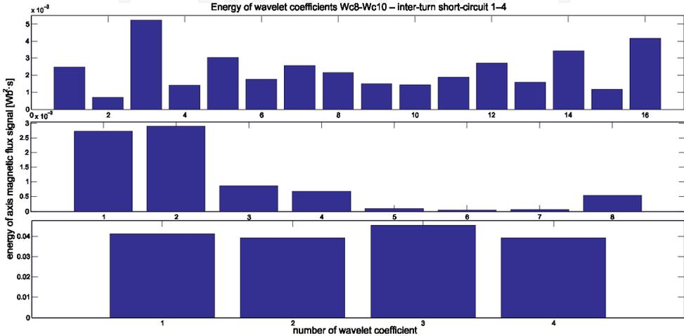
Fig. 11. Energy of wavelet coefficients of signal proportional to axial magnetic flux for the most important levels of wavelet representation from 8 to 10 – the case with inter-turn short-circuit type 1-4
