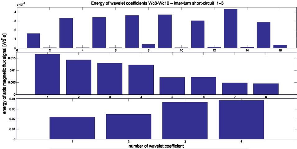
Fig. 10. Energy of wavelet coefficients of signal proportional to axial magnetic flux for the most important levels of wavelet representation from 8 to 10 – the case with inter-turn short-circuit type 1-3
