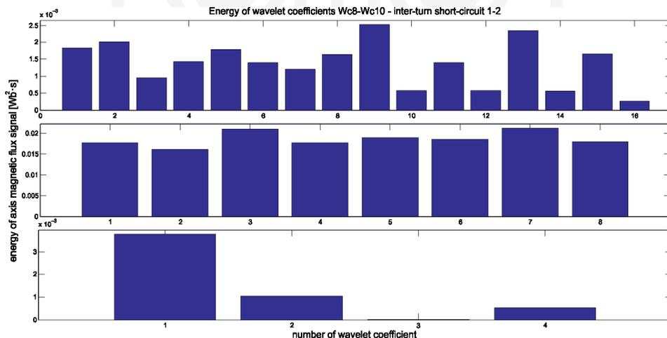
Fig. 9. Energy of wavelet coefficients of signal proportional to axial magnetic flux for the most important levels of wavelet representation from 8 to 10 – the case with the inter-turn short-circuit type 1–2
