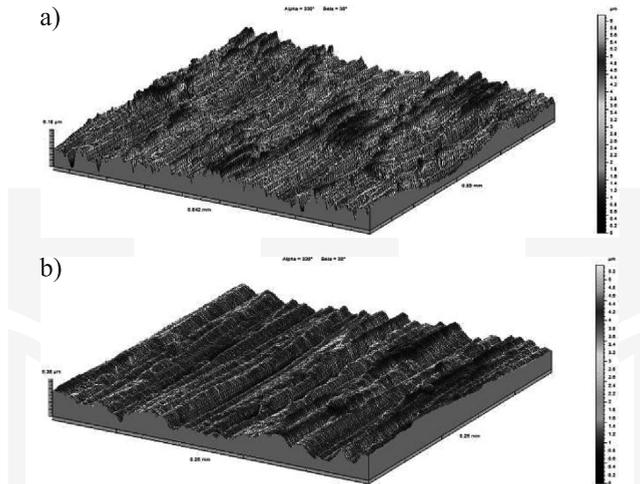
Fig. 2. The topography of borers flank after the fourth drilling cycle: isometric image (3D) of the studied surface (a) and enlargement of its selected fragments (b)
