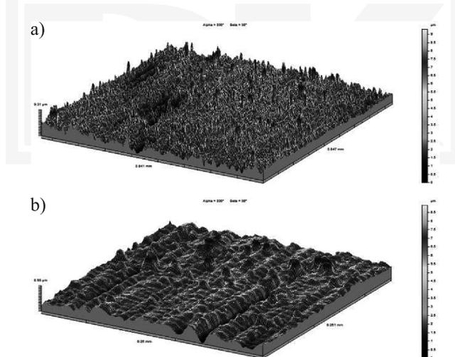
Fig. 3. The topography of borers flank after the fourth drilling cycle: isometric image (3D) of the studied surface (a) and enlargement of its selected fragments (b)
