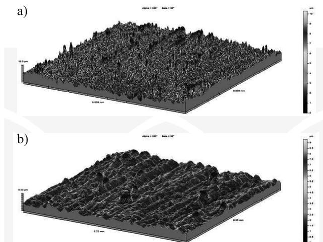
Fig. 4. The topography of borers flank after the fourth drilling cycle: isometric image (3D) of the studied surface (a) and enlargement of its selected fragments (b)
