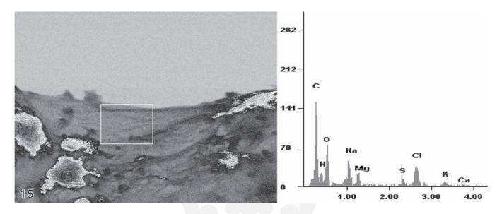
Fig. 15. Energy-dispersive X-ray spectrometric (EDX) analysis in the scanning electron microscope, using uncoated material. The analysed area of the *Eutintinnus angustatus* lorica is marked by a white frame ( $\sim 11 \times 9 \, \mu m$  in size). Since this part of the lorica was freely suspended in the vacuum, elemental detection occurred without influence of the carbon substrate.
