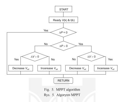
During its work power level and voltage of the PV system oscillates around maximum power point. This main idea of MPPT was developed but only in small range. For example in MPPT algorithm known as Perturb and Observe algorithm, perturbation coefficient is introduced. It decides about step size of the voltage changing during maximum power point searching process.
