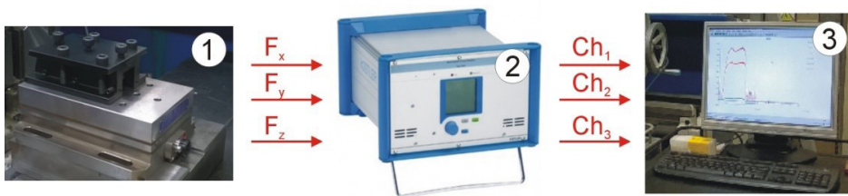
Fig. 1. The arrangement of measuring instruments to record the cutting forces of components:
