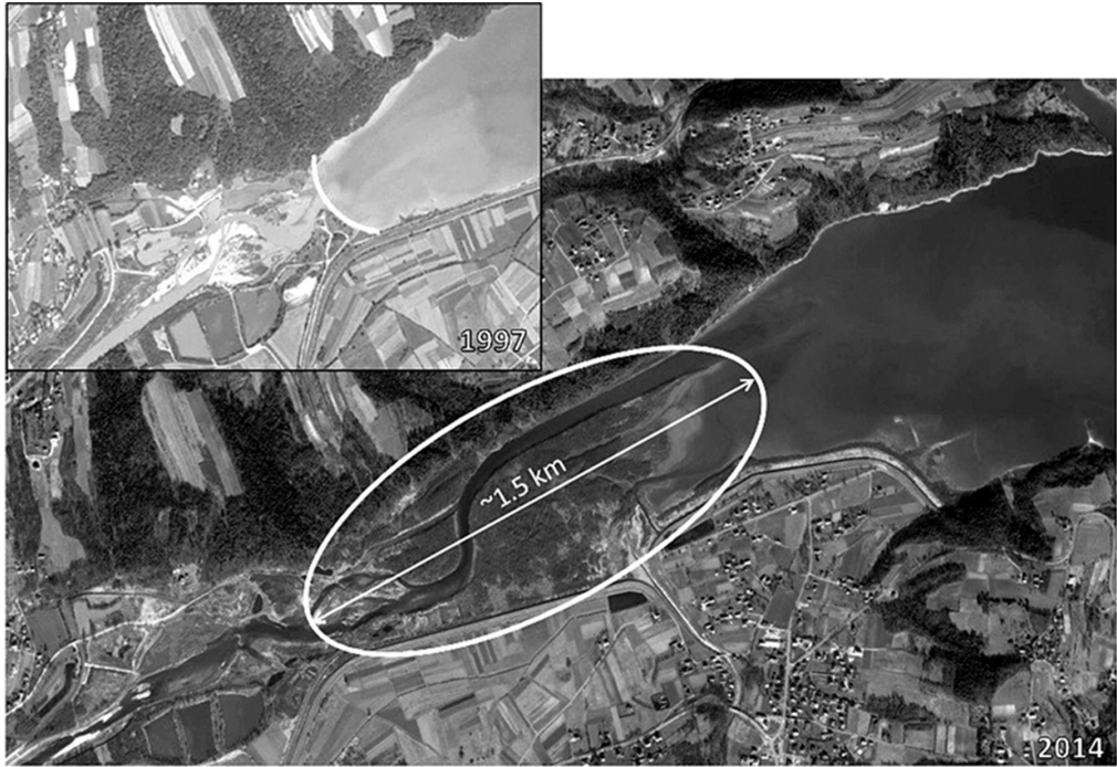
Fig. 4. Siltation of the backwater region 1997–2014
