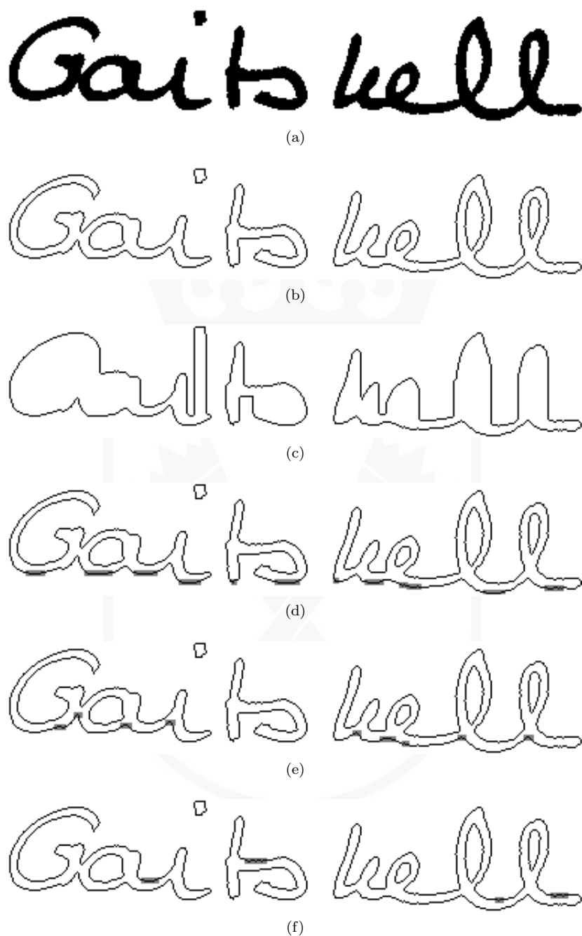
Fig. 4. Oversegmentation based on the word profile and contour. (a) An original image. (b) A word contour. (c) A word profile. (d–f) Potential split points: (d) lower contour minima; (e) lower contour maxima; (f) upper contour minima
