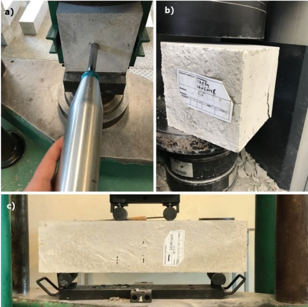
Fig. 4. Testing of the hardened concrete: a) sclerometric method; b) destructive test – uniaxial compression test; c) testing of concrete tensile strength under bending
